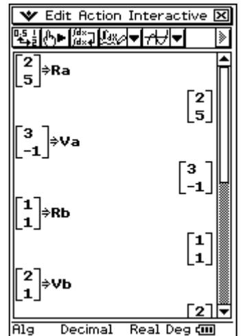
Next, create relative position and velocity vectors for A relative to B and store in **R** and **V**.
